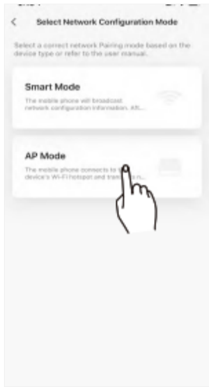
6.Click "AP Mode". Press and hold " " button on remote controller for 3~5s. After front panel appears "A2", click APP "confirm Indicator slowly blinks".
